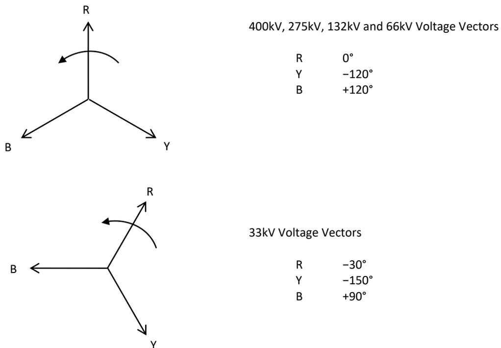
Figure 1: Northern Powergrid (Northeast) 132kV and EHV vector relationships
